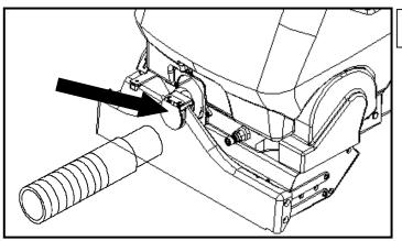
Lift door on front of vacuum shoe and insert 1 ½ inch hose cuff into hole.
